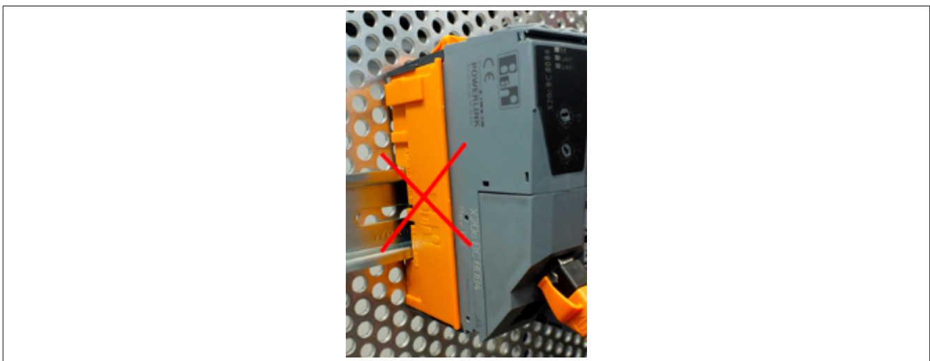
Figure 3: X20 system - Removing the end cover plates
