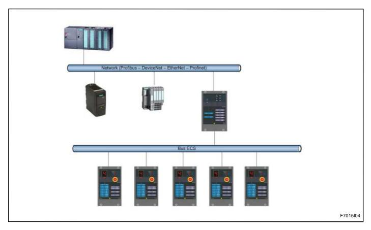
ESA BRIDGE is completely transparent in the data exchange, so it does not perform any management commands and states, leaving total flexibility of supervisor to manage the burners as needed.
