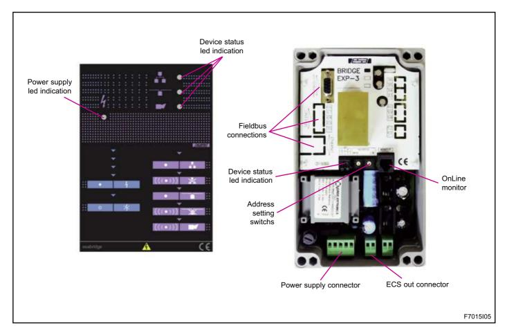
ESA EXP-3 is the reduced version of the device designed to be installed directly in the flame control when there are no other expansion cards. ESA EXP-3 has all the functionalities of ESA BRIDGE communication with the difference that it can only control one burner.
