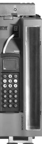
MDX60/61B application version for using "Electronic cam", "Internal synchronous operation" or the application modules.
