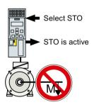
An active STO function prevents energy from being fed to the motor. The motor can no longer generate torque on the motor shaft.
