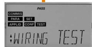
**TEST** to check inputs and to simulate outputs
