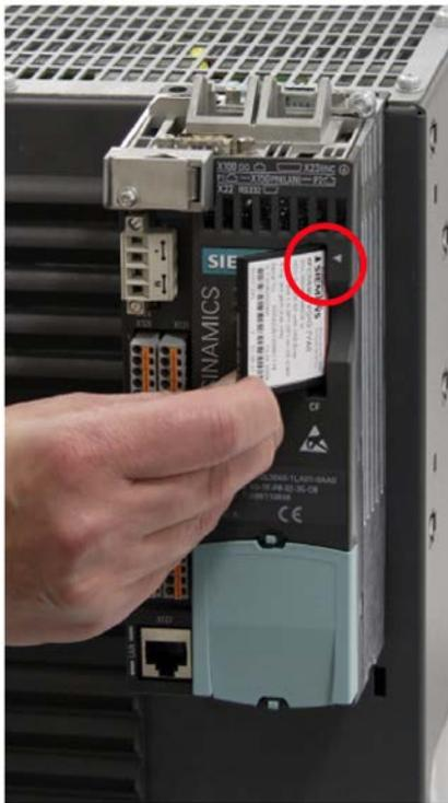
Figure 8-5 CU310-2 PN Inserting the memory card
