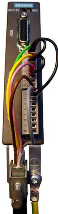
Figure 9-12 Photo of connection example 2: SMC30, 30 mm wide
