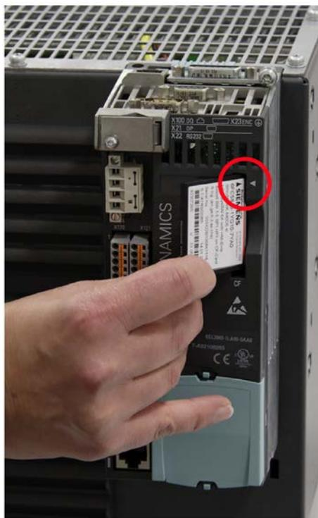
Figure 8-12 CU310-2 DP Inserting the memory card
