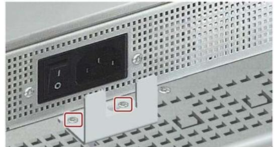
3. Insert the power cable into the socket and fasten the power plug fastener with the marked screws.
