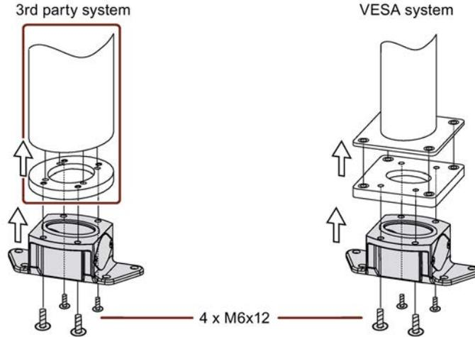
2. Attach the base adapter with 4 M6x12 screws to the mechanical interface of the support arm from below. Pay attention to the torque that is specified for the support arm.
