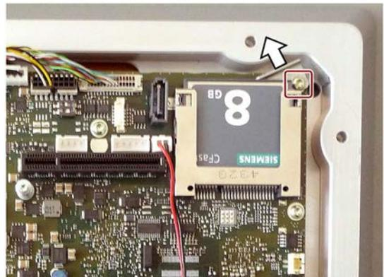
2. Press on the CFast card in the direction of the arrow.
