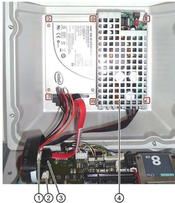
5. Remove the indicated countersunk screws on the back.
