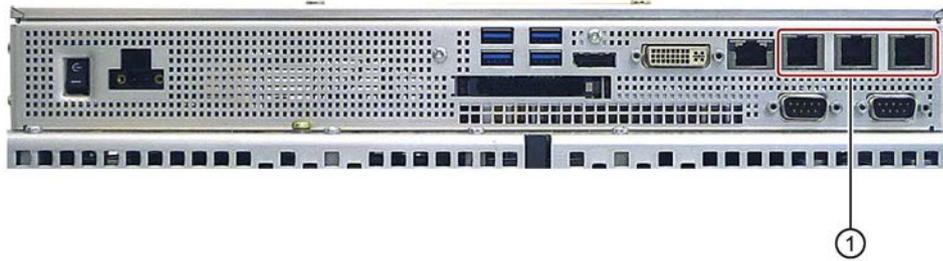
① 3 x PROFINET interfaces CP-1616 onboard ports via RJ45 socket
