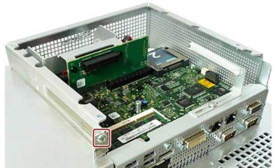
6.3 Removing a PCIe card (built-in units with PCIe card without DVD drive)
