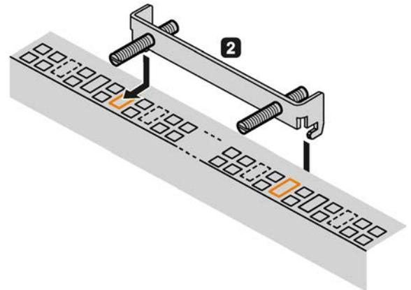
3. Secure the mounting bracket by tightening the threaded pins. The maximum permissible torque is 0.5 Nm.
