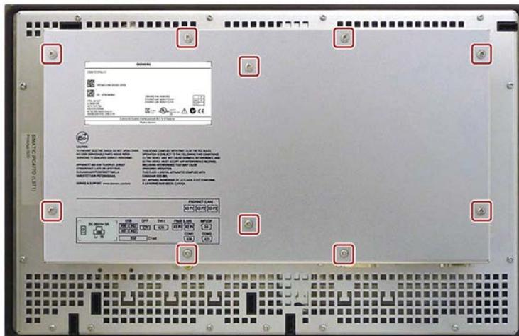
Position and number of the fastening screws are the same for the devices with 15", 19" and 22" display.
