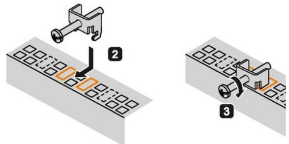
Mounting clips for devices with 15", 19" or 22" display
