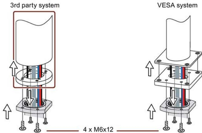
2. Insert all connection cables through the opening of the flange mount into the terminal compartment of the PRO device. Make sure that the connection cables are not damaged.
