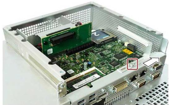
3. Insert the PCIe card in the direction of the arrow and secure this with the marked screw.
