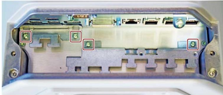
2. Connect the USB, DisplayPort and LAN cables.
