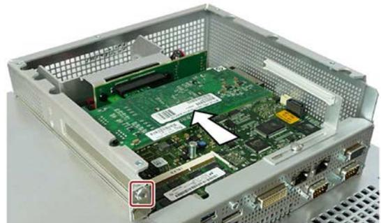
4. Push the PCIe card holder in the direction of the PCIe card and secure this with the marked screw.
