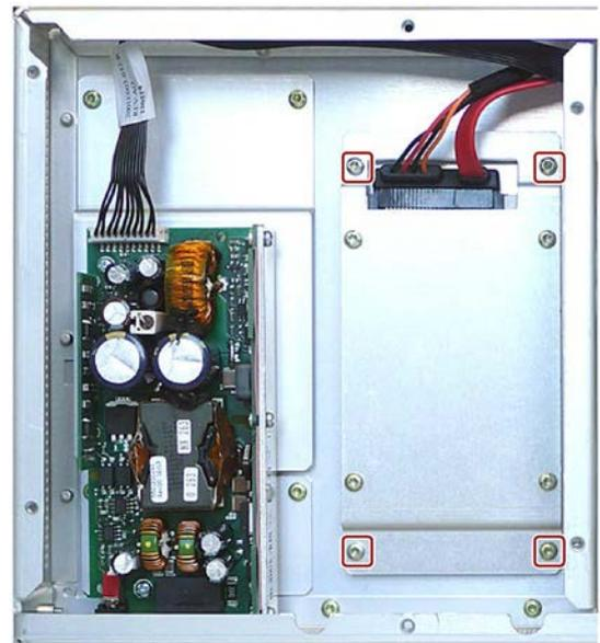
2. Remove the marked screws.
