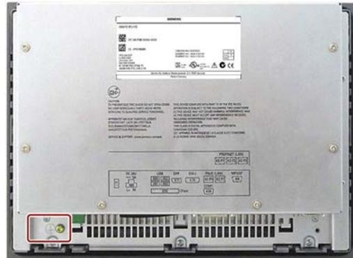
3. Connect the protective conductor to the protective conductor connection of the control cabinet in which the device is installed.
