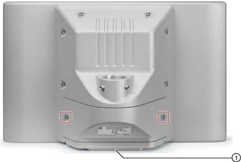
1. Loosen the indicated M4x16 screws.
