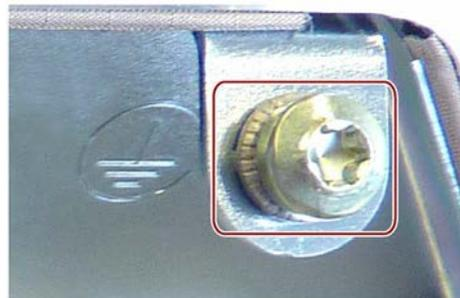
3. Connect the protective conductor to the protective conductor connection of the control cabinet from which the PRO device is supplied.
